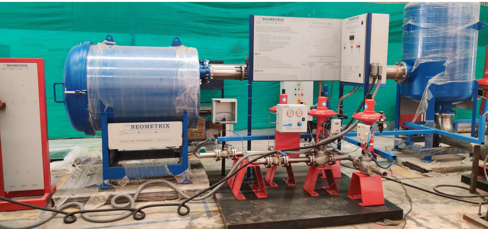
Aircrafts have varying atmospheric pressure conditions as altitude differs. We can create different altitude conditions inside a closed chamber by means of a vacuum pump and set of modulating and flow control valves. This Test Rig was designed for the ground testing of Aerospace Units. The test unit (UUT) will be placed between two chambers one of which is simulating cabin and other is simulating altitude chamber.
