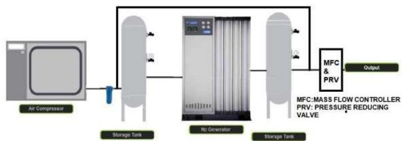
BLOCK LINE DIAGRAM OF Hypoxic Gas Generators (HGG-M-50LPM)
