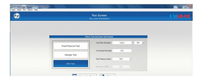
3. Choose the option of HSU TEST>enter Unit part number>choose LH or RH.>Unit serial number>test pressure (bar).Click OK. Below screen will appear.
