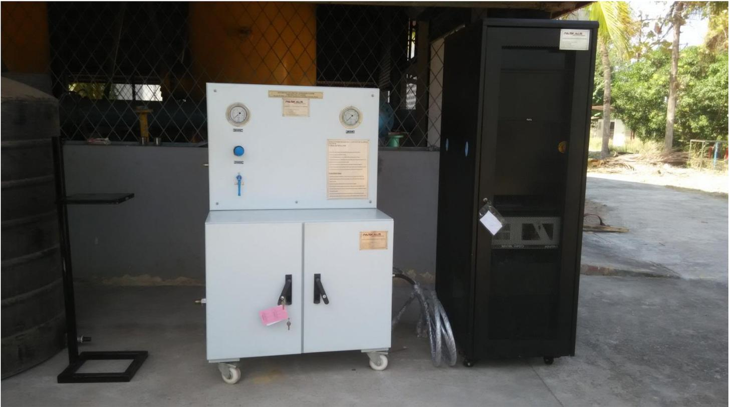
Hydrostatic testing is the most common method employed for testing pressure cylinders. Using this test helps maintain safety standards and durability of a cylinders over time
