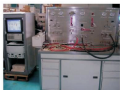
General Purpose Pneumatic Rig
