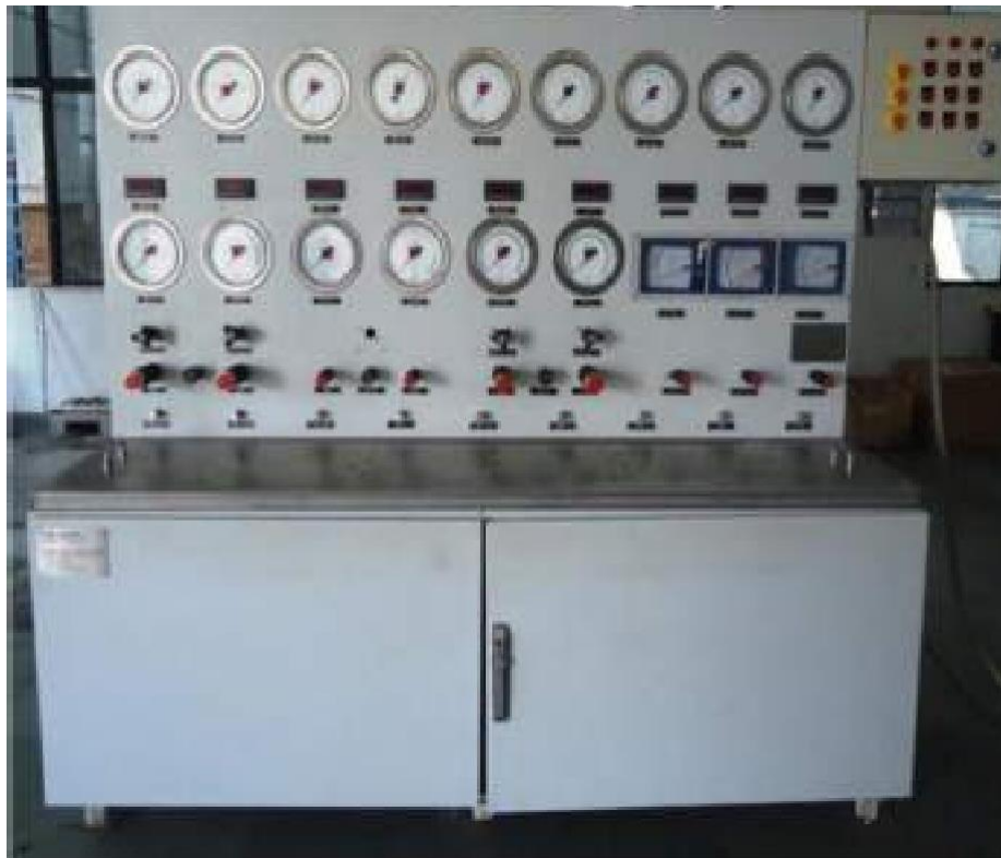
Control (USER) Panel of Component Test Rig for Flow/Cycling/ Pressure Test/ Flushing Applications
