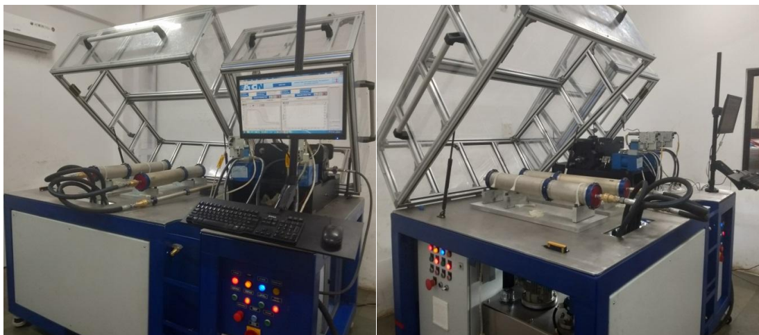
Impulse Test Section of the Test Bench (For Hoses, Flexible Pipes/ Tubes/ Fuel Lines)
