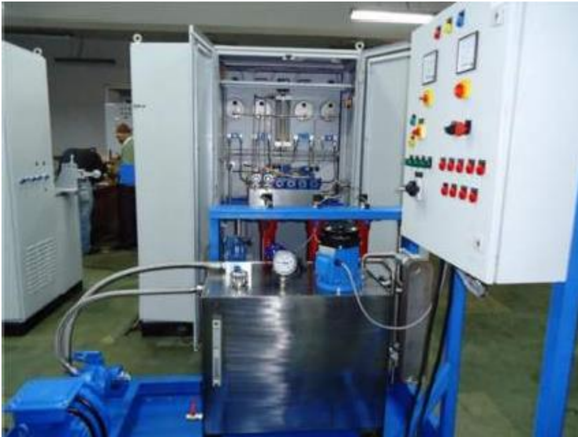
Hydraulic Power Packs designed for AVIATION applications. All pipelines/fittings /Tanks are SS 304
