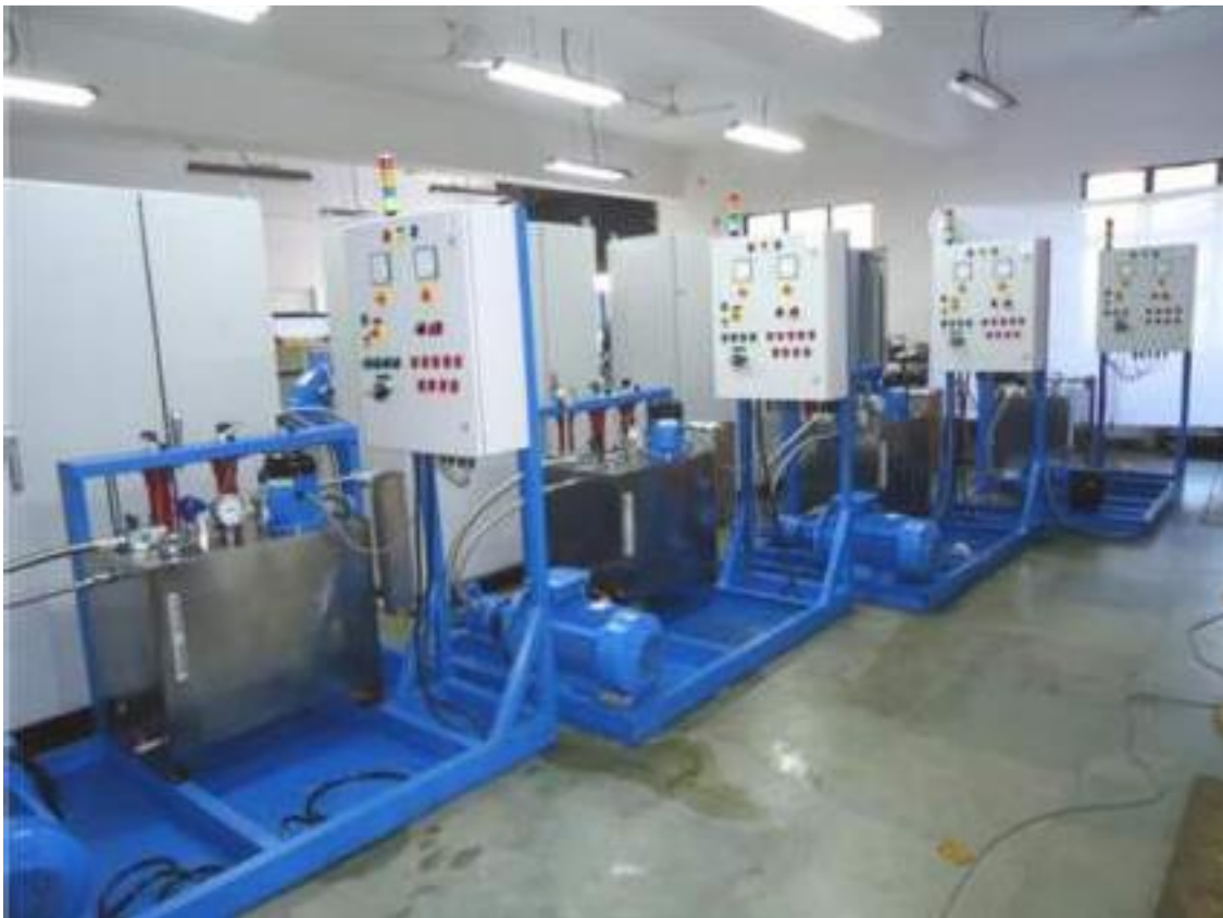
Hydraulic Power Packs designed for AVIATION applications. All pipelines/fittings /Tanks are SS 304
