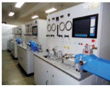
Servo Hydraulic Actuator Test Rig
