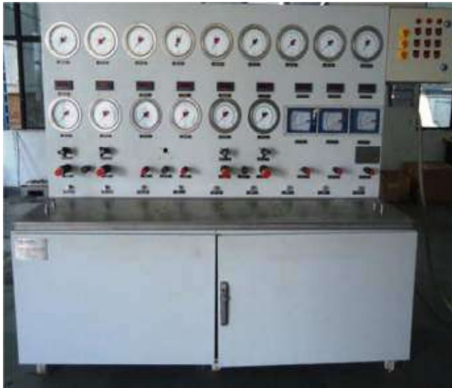
Control (USER) Panel of Component Test Rig for Flow/Cycling/ Pressure Test/ Flushing Application
