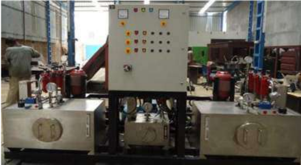
Hydraulic Power Pack of Component Test Rig for Flow/Cycling/ Pressure Test/ Flushing Application
