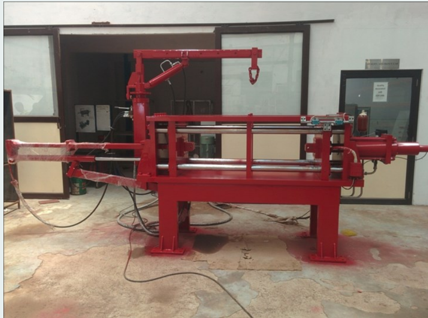
Snubber Test Rig
